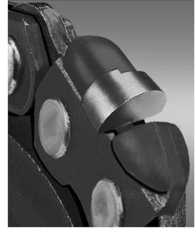
The BULLET® Chain is designed to allow chips of carbide to break away under normal use. **If 6 or more cutters (or 3 cutters in a row) have 50% or more of the carbide missing, the chain should be repaired.**
