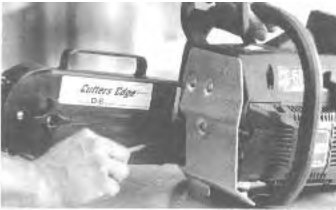
Fig. 17 Use the ball-driver to tension the chain.
