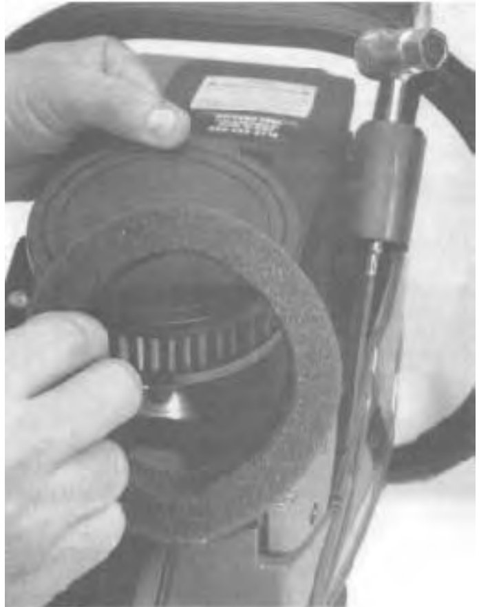
Fig. 34. Remove the pre-filter.
