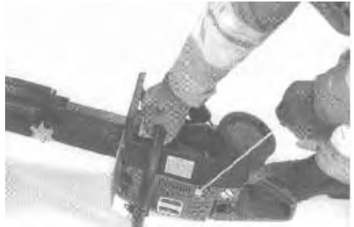
Fig. 12. Proper starting position.
