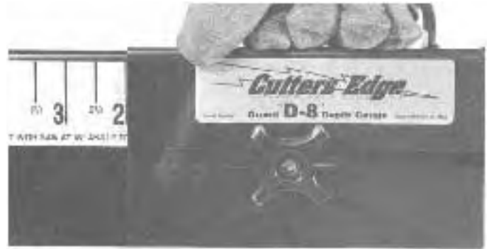
Fig. 18. Set the D-8 to the necessary depth.
