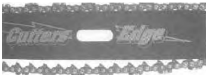
Fig. 14. The chain will sag when hot.
