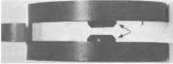
Fig. 16. Slip the spacers between two cutters.
