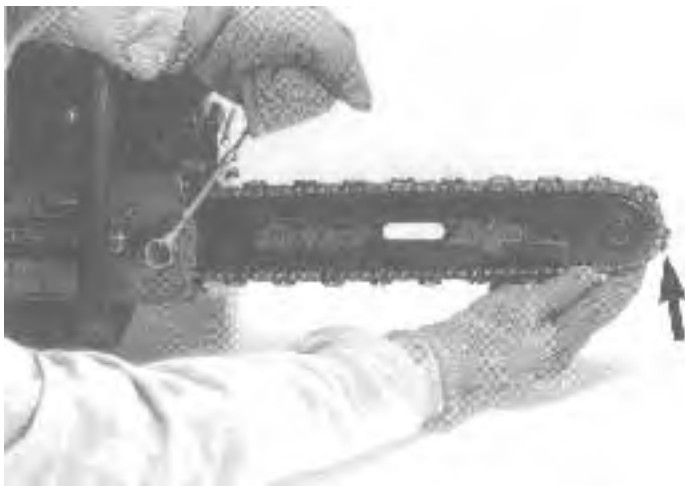
Fig. 9. Tightening the clutch cover nuts.
