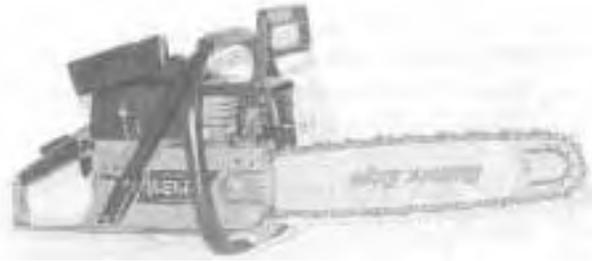
Fig. 31. Flip the guide bar each time you reassemble.
