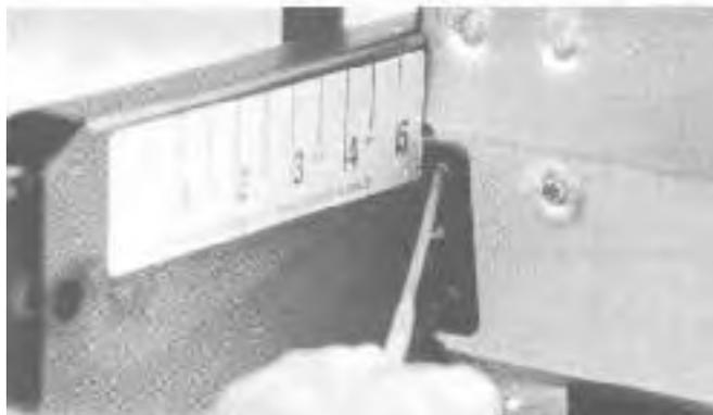
*Fig. 1. Use the ball-driver to tighten the alien-head bolts.*
