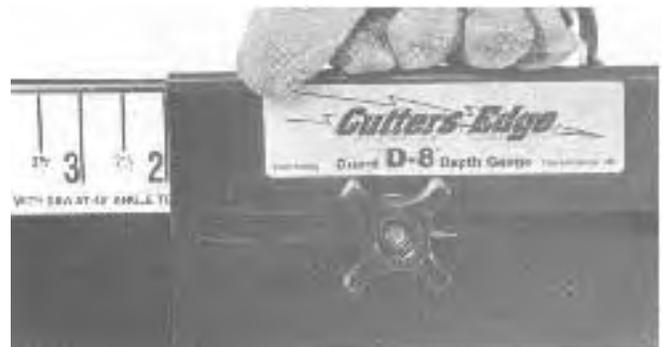
Fig. 6. Set the D-8 to the necessary depth.
