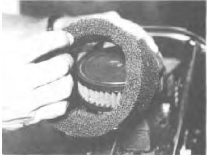
*Fig. 29. Remove the pre-filter.*
